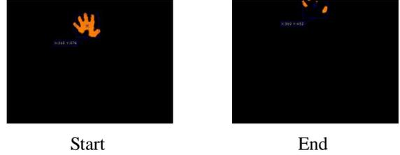
Figure 3. The starting and ending frame of a defected captured image showing hand movement to the top; after filtering. The center of gravity of the hand is also calculated despite most of the hand is not visible.
