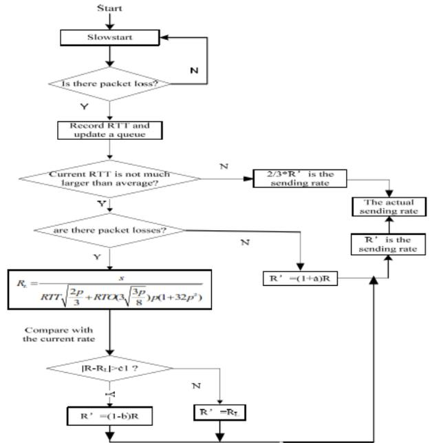
Figure 2: Flow chart for Transmission Control Mechanism
