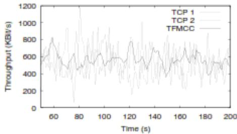
Figure 4: One TFMCC flow and 15 TCP flows over a single bottleneck
