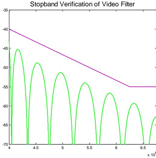
Figure 2: Video Filter Stopband
