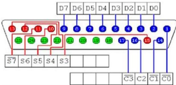
Figure 2. Parallel port connectors
