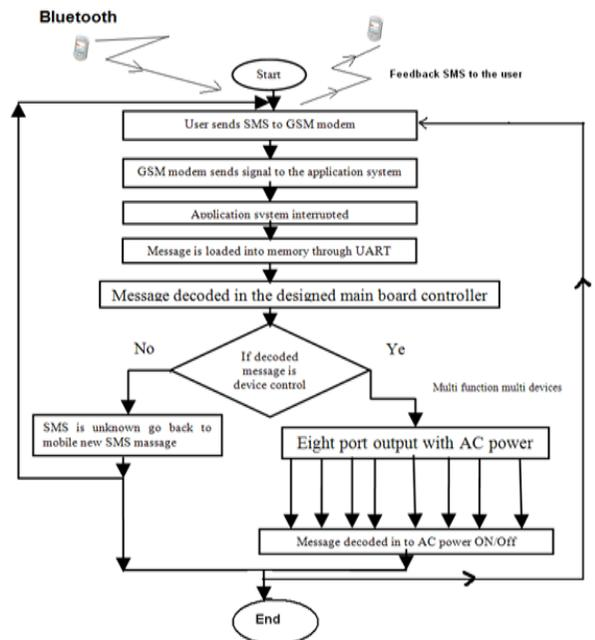
Figure 4. System methodology and application system
