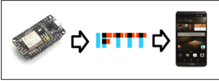
Figure 3. Sending a message from the circuit to Mobile via IFTTT.com.
