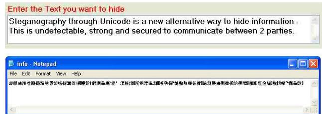
Fig. 2 Text File contains Original message hidden through Unicode Symbols
