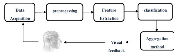
Figure 2. Functional Model of a BCI System. The signals are obtained by a signal acquisition system, processed by signal enhancement methods and classified in a specific BCI application.
