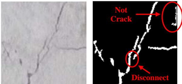
Fig2. A result of the detection method using wavelet transforms [7]
