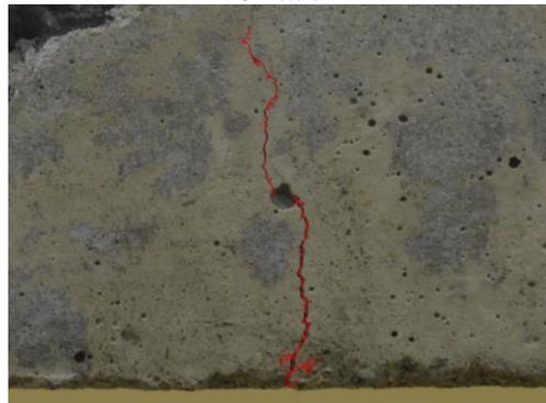
Fig12. a detection result image from the distance of 3 meters
