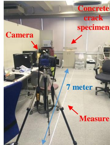
Fig10. The shooting scene of the concrete crack specimen
