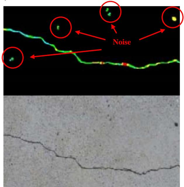
Fig3. A result of the detection method by the probabilistic relaxation method using line emphasis [9]
