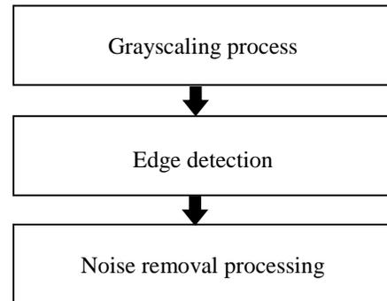
Fig4. A process flow of the V-shaped detector
