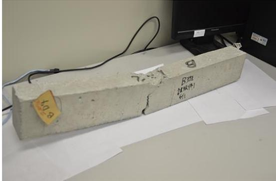
Fig7. Concrete crack specimen
